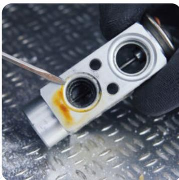
**Impurities and debris concentration inside the TXV.** System contamination, additives, worn receiver-dryer, particle formation after AC compressor seizure, improper flushing - all these may lead to inner blockages of the valve.
