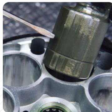
**Severe AC compressor failure > seizure.** Impaired lubrication caused by overheating, lubricant dilution or excessive impurities formation. All can be linked with a faulty TXV.
